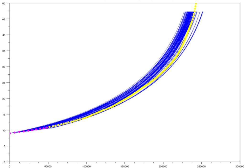
Forecasting for crack 2 (no jump model)
